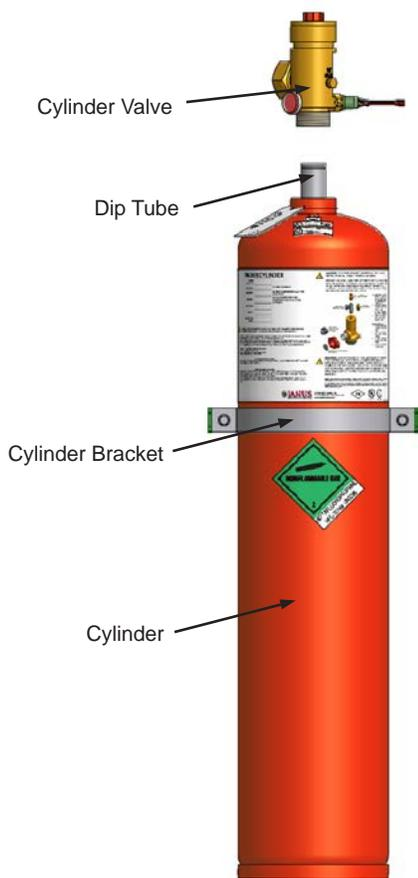
**Cylinder Valve:** The automatic release of FM-200<sup>®</sup> is controlled by a forged brass, differential pressure operated cylinder valve connected to the neck of the cylinder. The valve assembly is shipped with an anti-recoil safety plug installed in the discharge outlet and chained to the cylinder valve.
