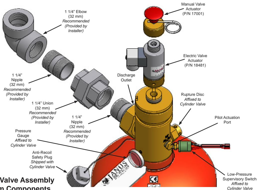
**Cylinder Valve Assembly with Trim Components**
